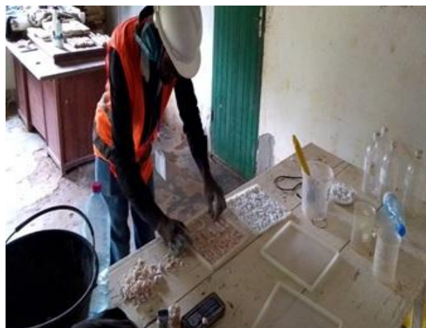
Fig. 4. Placing and arrangement of marble's aggregates in a mold for tile processing.
