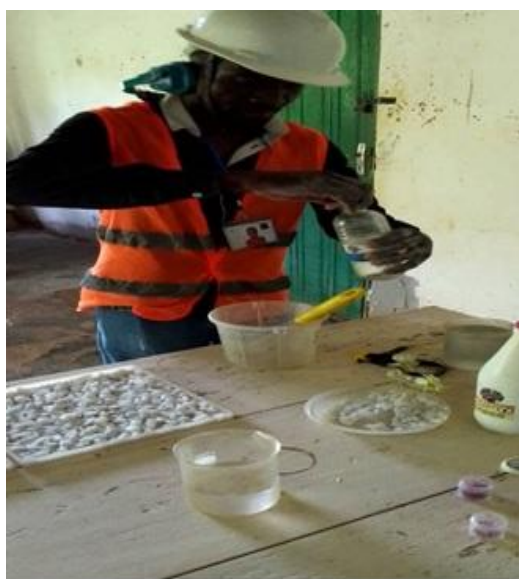
Fig. 3. Preparation of epoxy resin mixture during the processing of the tile.
