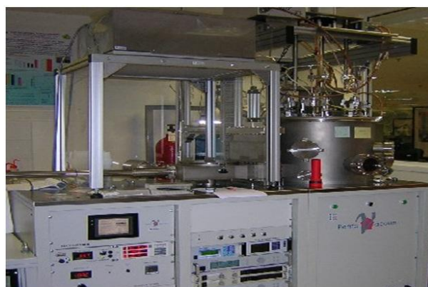
Fig. 1. Photo of an unbalanced magnetron sputtering deposition system used in this study.
